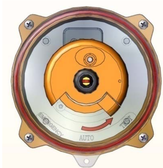
Figure 7 Indicator Beacon Selftest (TEST)
